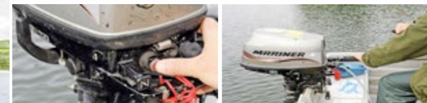
The shift lever (far left), choke and stop button (under thumb) are easily located. Sit down when starting the engine and be patient if it doesn't start first time.
